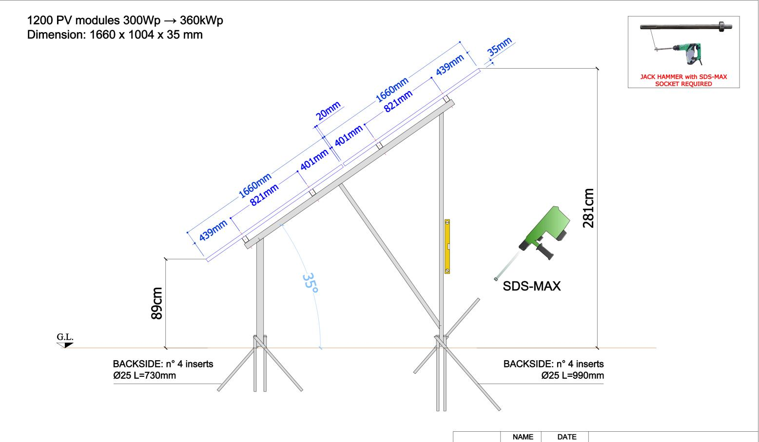
Driving-in the inserts to the ground through guides placed at the base of the frames, using a jack-hammer with SDS-MAX tool tip or a common hammer, only when all the structure is installed and it has checked that the spirit level giving the transverse orientation of the structure indicates the horizontal.
